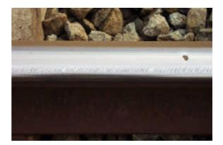
Figure 1: Headchecks at gauge corner
