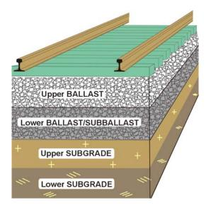
Figure 1: Idealized track substructure.
