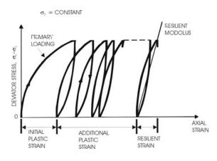
Figure 2: Cumulative Strain and Stiffness of Materials Under Repeated Loading
