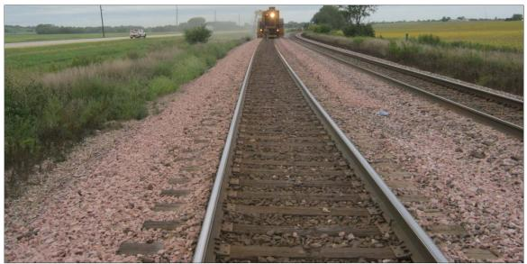
Figure 25. Test Site before Ballast Shoulder Cleaning Note. New ballast (pink colored) along both ballast shoulders
