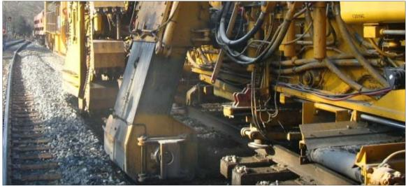
Figure 7. Track Undercutting<sup>3</sup>
