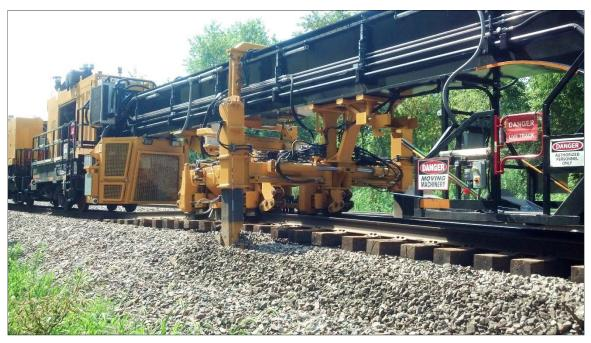
Figure 10. Loram Track Lifting Machine<sup>5</sup>
