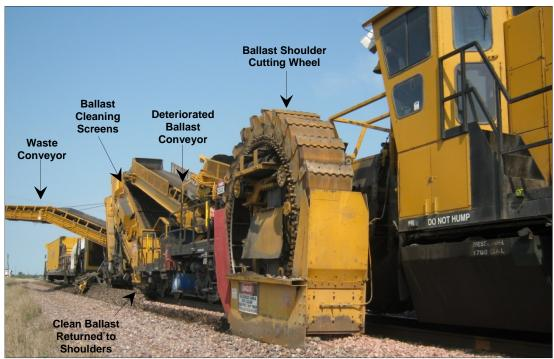
Figure 24. Details of Loram Ballast Shoulder Cleaning Operation Note: Machine is symmetrical and cleans shoulders on both sides of the track simultaneously
