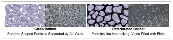
Figure 2. Comparison of Clean and Deteriorated Ballast
