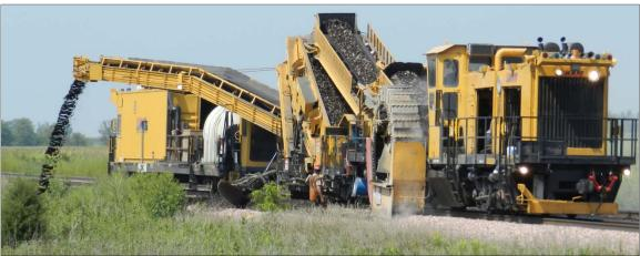
Figure 23. Loram Ballast Shoulder Cleaning Consist
