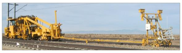
Figure 3. Track Surfacing and Alignment Machine
