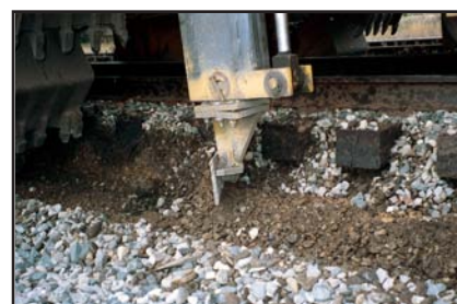
Scarifier tooth. A scarifier tooth on each side of the machine undercuts the tie ends up to 5 inches (125 mm) to break up mud pockets and restore drainage.
