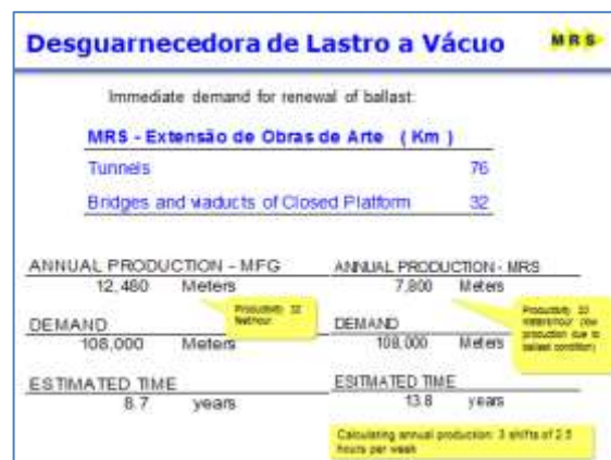
Figure 3: Estimated time for entire Specialty Trackworks System Ballast Remediation with Traditional Method (right side) and with Loram's Railvac (left side)
